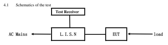
EUT: Equipment Under Test
